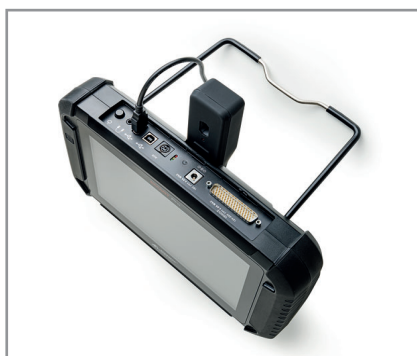
The Smart Programmer connects to the rear of the Smart Pro via the USB cable
