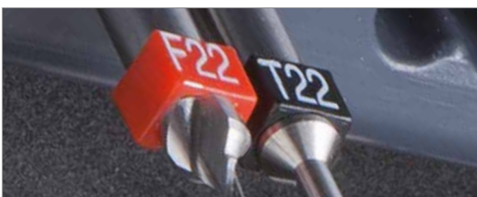
Cutting tools with identification collar
