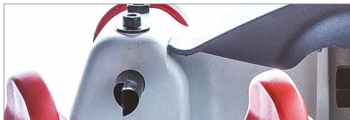
Tracer point with micrometric adjustment
