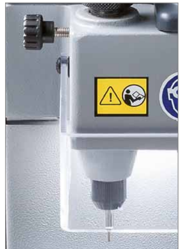
Spring loaded tracer point
