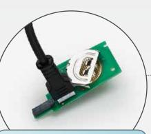
2. Connect the Universal Remote Cable to the Universal Remote Car Key. Make sure the battery is removed from the PCB during the pre-setting.
