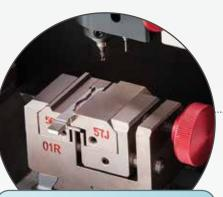
**5.** MySilca SRP app tells you what CH blade you should use. Cut the CH key blade with a Silca key cutting machine.
